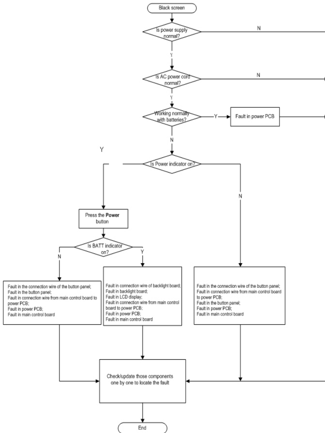
Figure 4-7 Location flow of faults causing black screen
